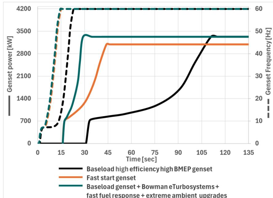
Comparing to the NG ICE fast start version that can fulfill grid balancing and datacentre back up power requirements globally today, the addition of Bowman eTurbo systems to todays best in class baseload versions offers the potential to achieve site level:
