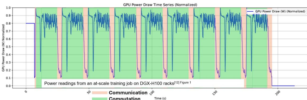
The peak-to-peak power swings of 80 to 90% of TDP seen at GPU level, translate to peak-to-peak power swings in the region 50 to 60% of the entire datacentre site (reduced versus rack level by ~1/3 reduction as the GPU's are not the only onsite electricity consumer), inflicting significant strain on the local grid infrastructure. Within the computation phase, the high frequency oscillations typically seen in GPU operation are similarly reduced at datacentre level to ~15% peak-to-peak.
