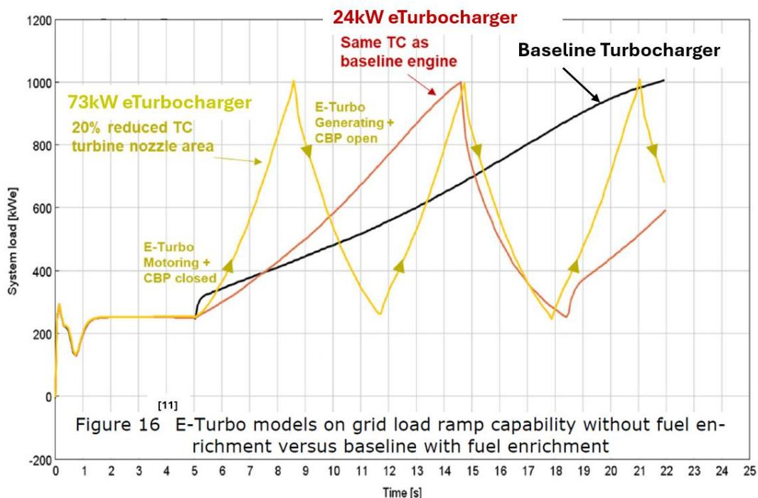
Figure 16 E-Turbo models on grid load ramp capability without fuel enrichment versus baseline with fuel enrichment
