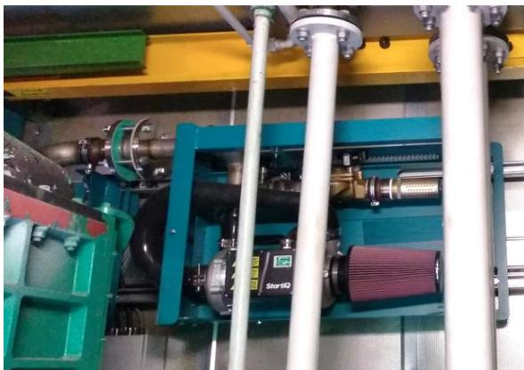
genset platform was able to reliably achieve start command to 100% load (with the genset in cold, pre-heated condition) in less than 60s, as per the 'Time to full delivery' PQR requirement. In each case, the cumulative fuel consumption, CO<sub>2</sub> and NO<sub>x</sub> emissions were reduced by 80 to 90% during the load ramp phase.
